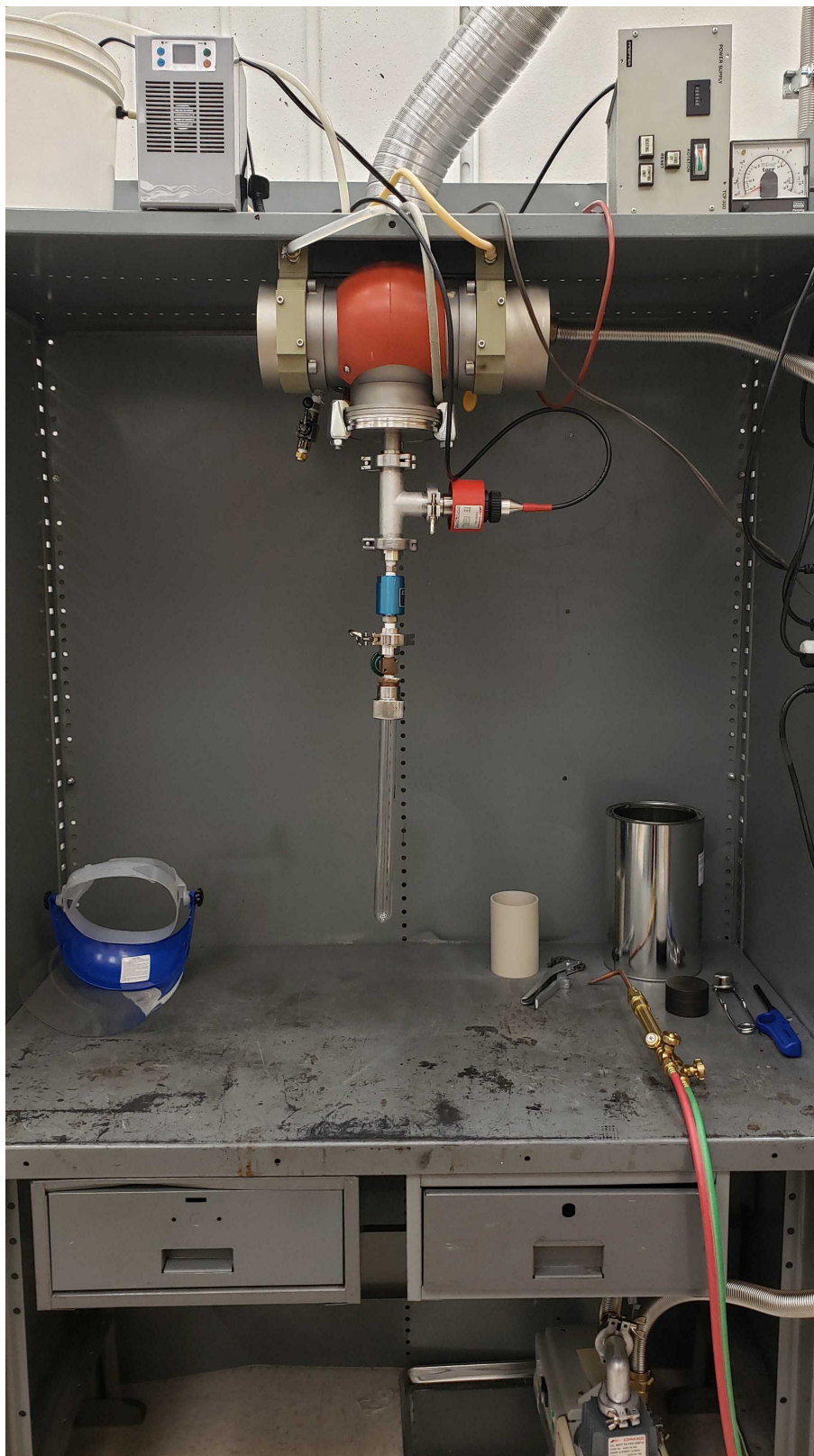
Figure 3.1 Photograph of the vacuum sealing system used for the synthesis.
