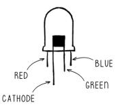
Let's connect the RGB to our Arduino so that we can separately control each of the colors emitted by the LED. We'll start with the circuit itself.
