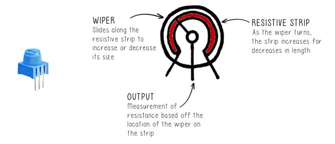
The input voltage is applied across the whole length of the resistor, and the output voltage is the voltage drop between the commencing point and the point where the sliding contact lays.
