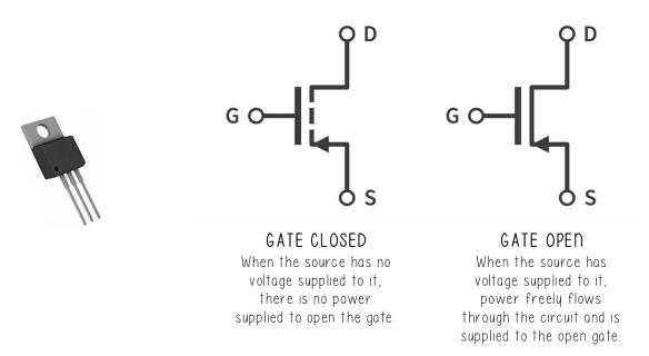
Metal-Oxide-Semiconductor Field-Effect Transistor (MOSFET)
