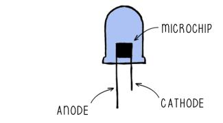
As an electrical current passes through the microchip, it illuminates and creates the visible light that we identify as a light-emitting diode (LED). The long pin, called an anode, is connected to power or a voltage supply whilst the short pin, called a cathode, is connected to negative or ground. Current in an LED flows from the anode to the cathode and never in the opposite direction.
