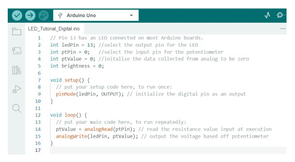
Carefully (ever so slightly) twist your potentiometer to see how the LED reacts. As we slowly turn the potentiometer, the LED can be seen to have its brightness determined by the analog input by the analog output.
