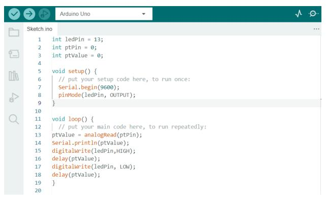
Upload your code to the Arduino and open your serial plotter on the top right of the Arduino IDE.
