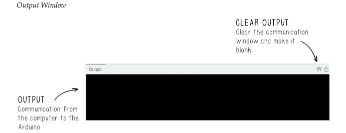
Output – communication between the computer and the Arduino. This window will declare success or may display any errors present during compiling and/or uploading.
