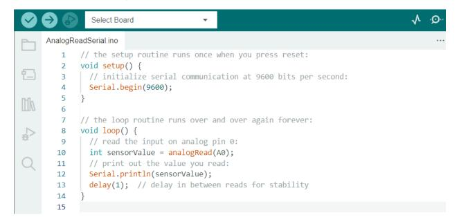
Serial. begin(), Line 4 – Initializing the serial communication. By initializing the serial communication, the user can access the input data from the Arduino board in real-time using the serial monitor or serial plotter in the Arduino IDE. The format to initialize the serial communicator is as follows:
