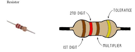
A resistor is a passive two-terminal component that limits the current flowing through itself by creating resistance through heat. The resistance of the resistor is determined by a ceramic rod wrapped with a copper wire – the thinner the copper wire, the higher the resistance, and the same stands for a thicker wire having a lower resistance. The colored bands on a resistor demonstrate the resistance of the resistor. The table below explains each color's meaning and representation:
