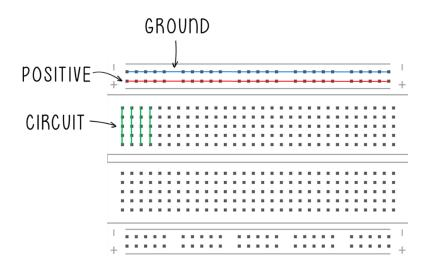
A breadboard is a plastic board with interconnected pins that are used to connect electrical components to create a functional circuit. There are two kinds of strips – bus or power strips and terminal strips. Terminal strips (green) are used to connect the electrical components, each strip is connected vertically but not horizontally. Bus or power strips (red and blue) are used to connect power or ground to the terminal strips, these strips are connected horizontally to one another.
