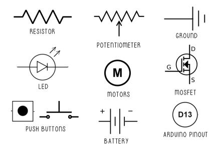
All electrical circuitry is described through universal electrical symbols – they are a graphical representation of circuits. Think of it as a universal language. All circuits start with a symbol and end with a symbol and all symbols in between are connected with plain lines.
