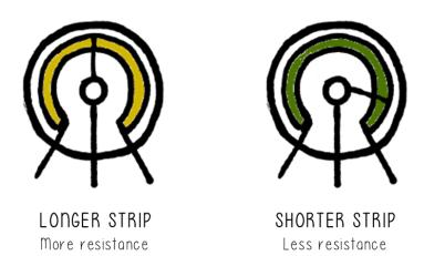
As the dial on the potentiometer is turned, the position of a sliding contact wiper across the resistance strip changes and therefore, increases or decreases the total resistance.
