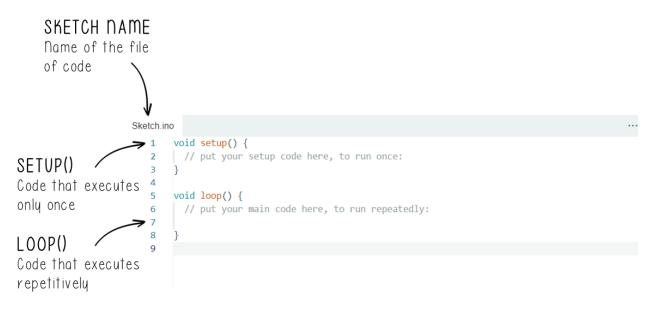
Setup – the sketch's starting point. This is where variables and pin modes should be initialized as well as accessing libraries, etc. The setup function will only run once and will re-initialize each time the Arduino is powered up/reset.
