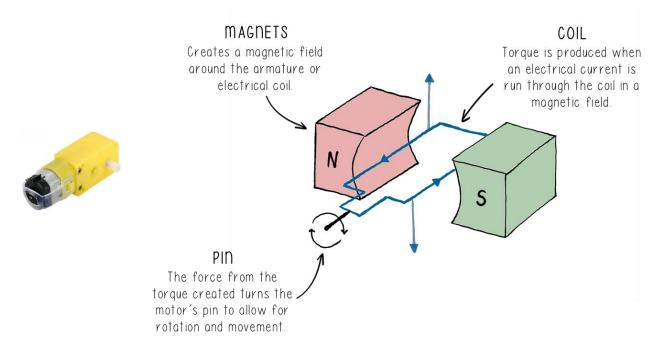
DC motors take electrical power through a DC current and convert the energy into torque and mechanical rotation within the motor. Within the motor, magnetic fields are created to allow an electrical coil to rotate when an electrical current is running through it. When the two interact, the torque created generated the mechanical rotation of a pin.
