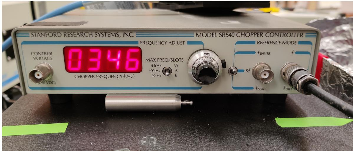
**Figure A.9** The chopper's control box.
