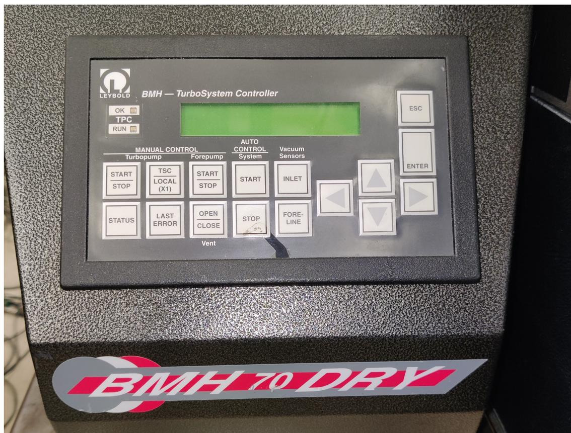
**Figure A.3** The vacuum pump. Only ever touch the power switch and Auto Control System Start/Stop.
