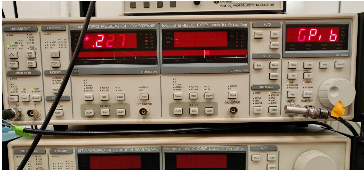
Figure A.7 The lock-in amplifier.
