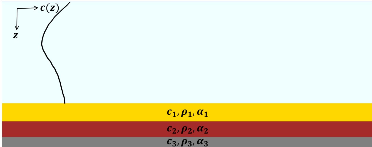
Figure 1.6 Simplified version of Fig. 1.1 representing the parameterization used in the range independent normal mode model ORCA [2].
