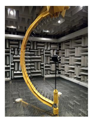
**Figure 15.8** Directivity measurement system assessing the radiation of a spherical loud-speaker positioned at its center. The white disc controls the aperture size.
