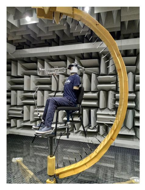
Figure 11.2 Directivity measurement system with an artificially excited trumpet and manikin.
