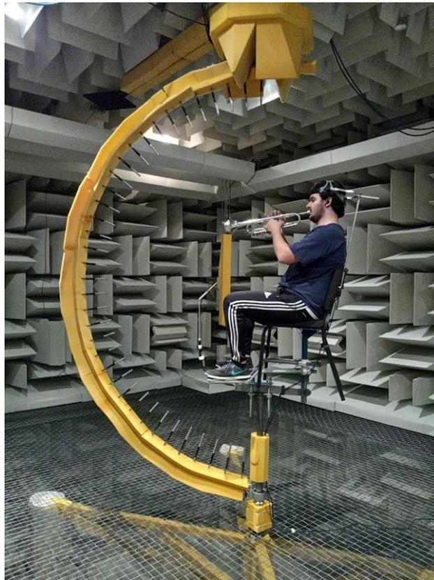
**Figure 3.5** Trumpet player within measurement arc while playing with a cup mute.
