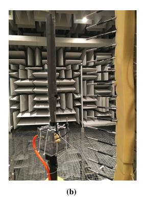
**Figure 13.1** Spherical (a) and cylindrical (b) microphone arrays used to assess the radiated fields of two organ pipes.
