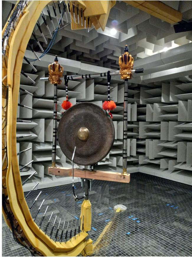
**Figure 8.1** An ageng lanang gamelan gong within the rotating directivity measurement array.
