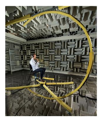
**Figure 7.1** A microphone array used in measuring spherical directivities of musical instruments and speech. The array has  $5^{\circ}$  resolution in the polar angle. A full spherical directivity follows by rotating the musician or talker in  $5^{\circ}$  azimuthal steps and using a transfer function technique to address repetition variations.
