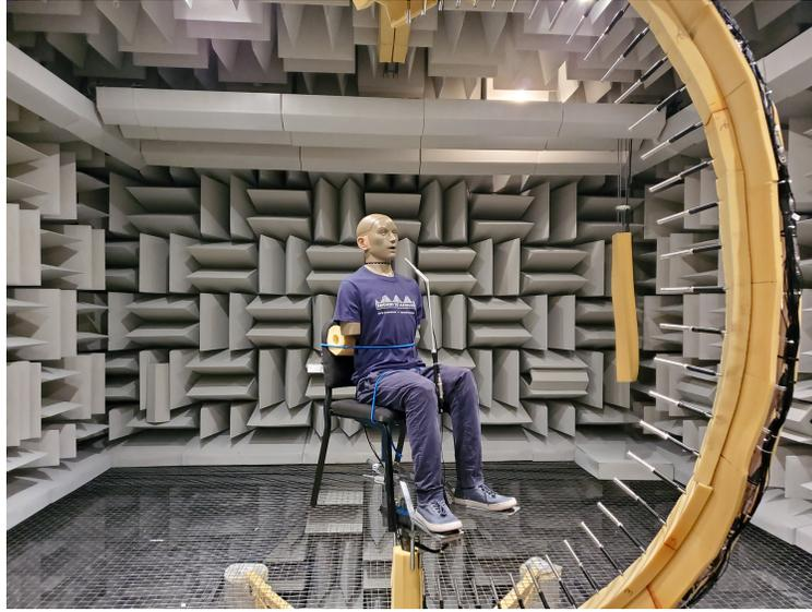
**Figure 1.10** KEMAR HATS seated within a directivity measurement system.
