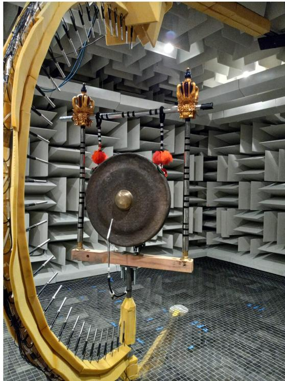
**Figure 14.1** An ageng lanang gamelan gong within the rotating directivity measurement array.
