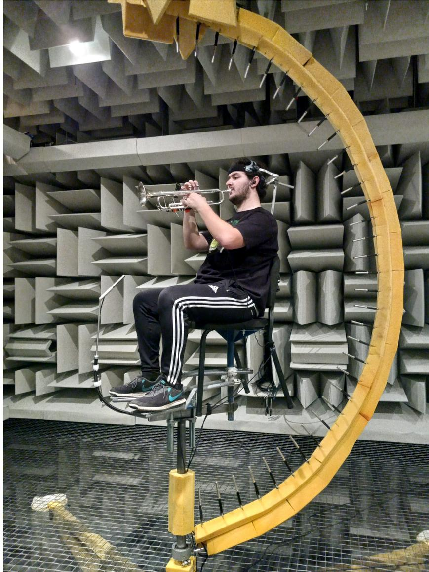
**Figure 11.1** Directivity measurement system with a musician and trumpet.
