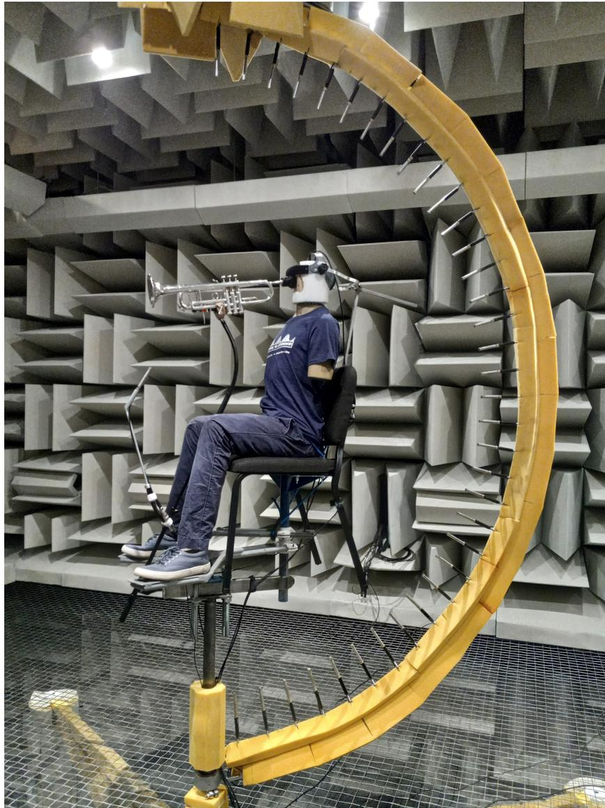
**Figure 11.2** Directivity measurement system with an artificially excited trumpet and manikin.
