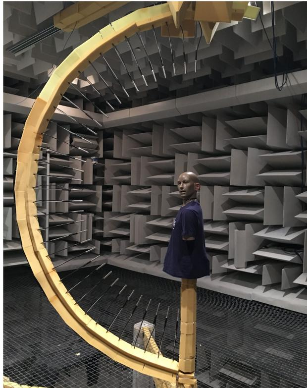
**Figure 10.1** A KEMAR HATS within the rotating directivity measurement system.
