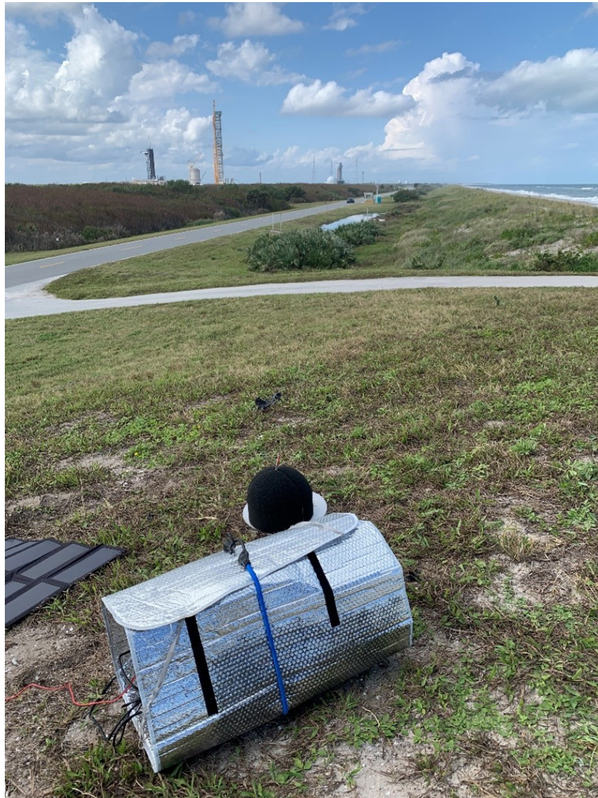
Figure 1.2 View from the data collection station, Station 02, shown along the coast 4.1 km from the launch pad. The Space Launch System can be seen in the distance near the white dome. Stations include data acquisition devices, under the reflective covering, a solar panel, and microphones that are shielded by a wind screen.
