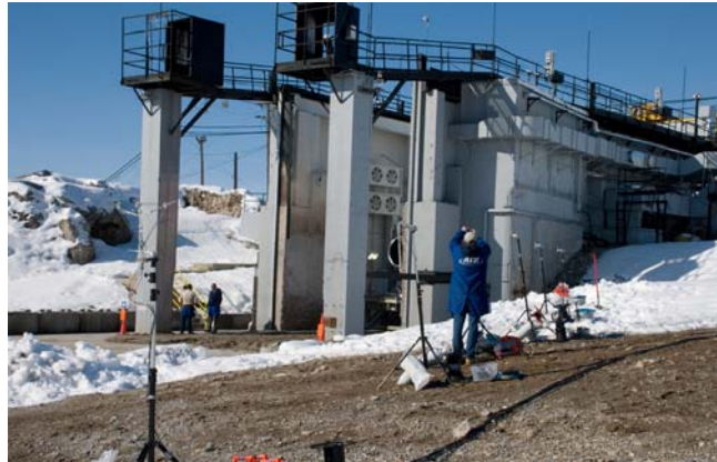
Fig. 3. (a) View of the GEM-60 Solid Rocket Motor during a static test. The brighter part of the plume is approx. 150 feet in length. (b) GEM-60 test bay with tripods aligned along the plume. The gentleman in the picture marks the location of the temperature probe and 1/8" microphone.
