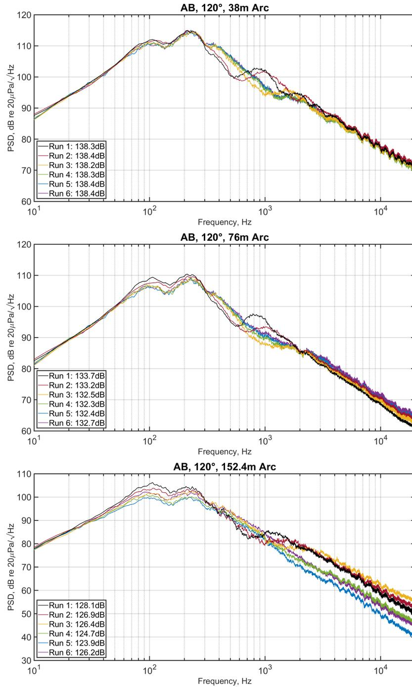
**Figure A.2** Comparison of runs at 120° for the three arcs at afterburner (AB)
