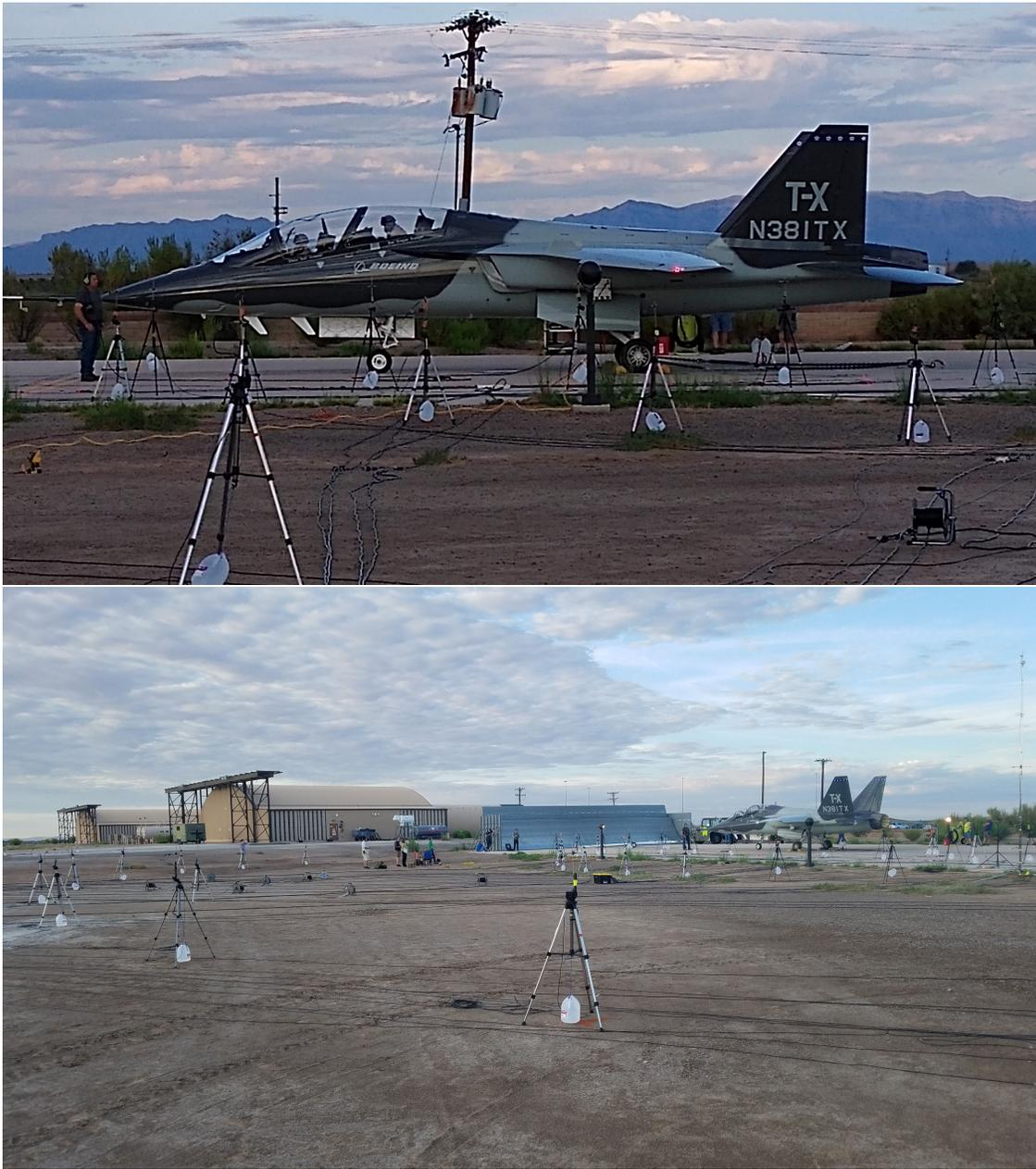
**Figure 2.1** The T-7A from the side view and the 38 m (125 ft) arc around the aircraft.
