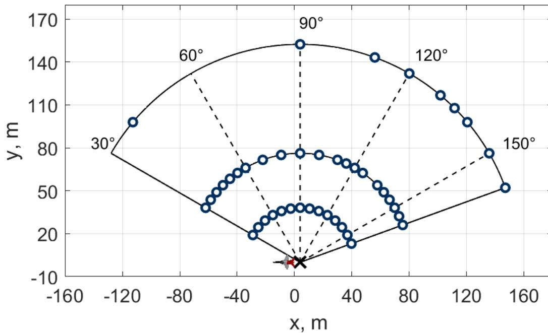
**Figure 2.2** Representation of the microphones and their positions on the 38 m (125 ft), 76 m (250 ft), and 152.4 m (500 ft) arcs.
