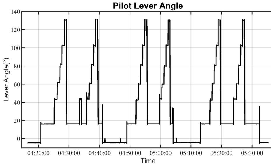
**Figure 3.3** Pilot lever angle during the measurement. Each step during the six runs indicates the next engine condition lasting about 30 seconds.
