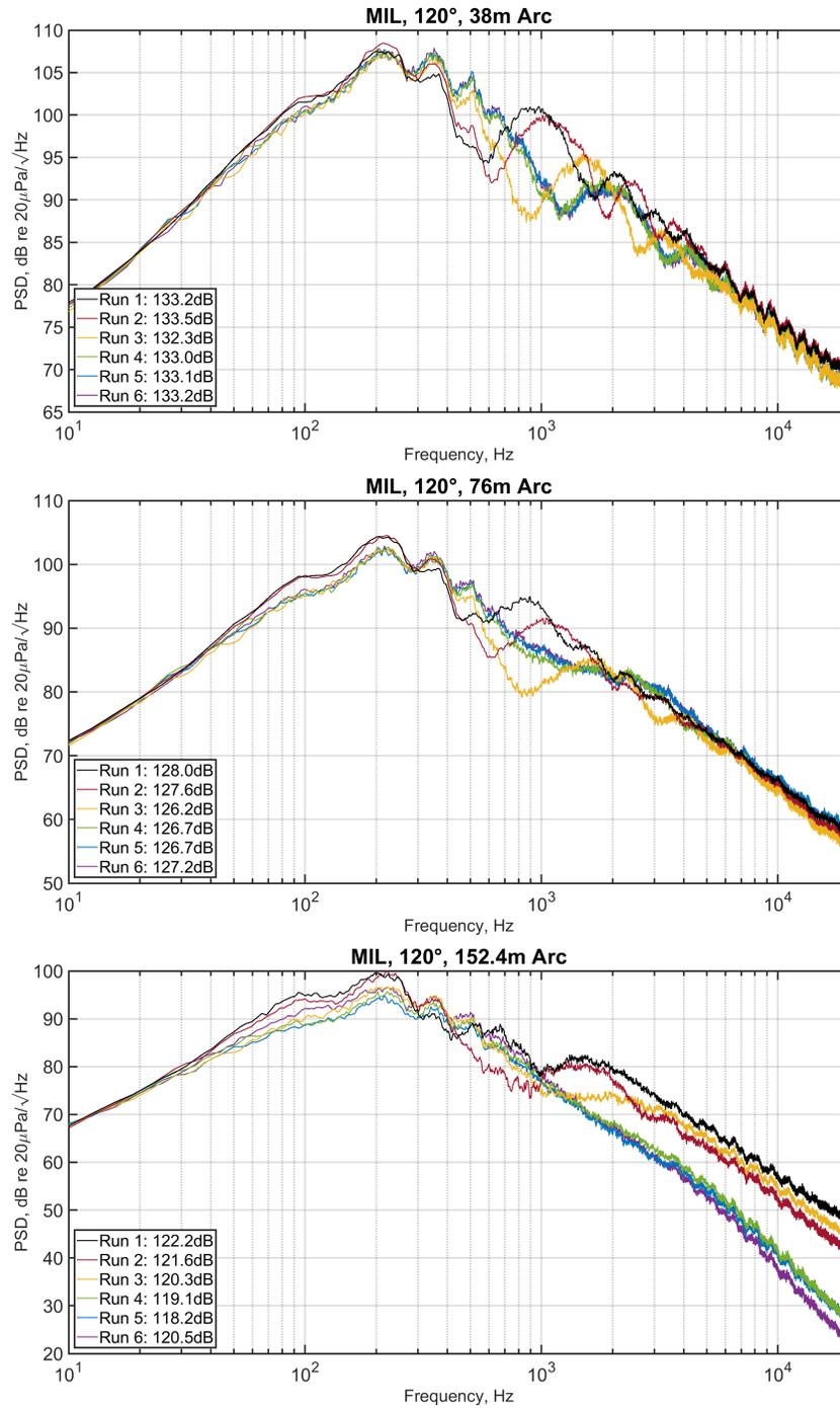
**Figure 3.2** In contrast to the last set of graphs, these depict a comparison of runs at 120° for the three arcs at military power (MIL)
