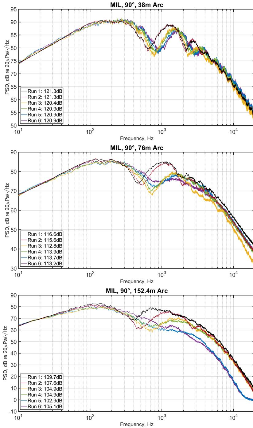
**Figure A.1** Comparison of runs at 90° for the three arcs at military power (MIL)
