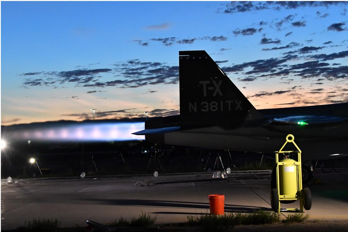
**Figure 1.1** Full Afterburner of the T-7A during the run-up. Due to the high temperature and speed of the emitting gases, they remain together farther downstream.
