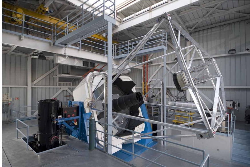
Figure 2.1 3.5 meter telescope located at Apache Point Observatory. The observing mirror collects the light and focuses it onto the secondary mirror centered in front of the mirror. The large metal structure directly in front of the observing mirror are the lamp lattices used to take calibration images.
