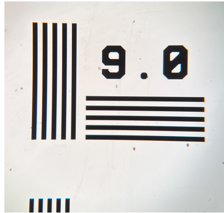
Figure 3.1 The US Air Force resolution test chart as imaged with a visible light microscope with back-lighting. The number "9.0" here represents 9 lines per millimeter, and the five lines visible at the bottom left are the lines belonging to the 10 lines per millimeter pattern below. There is slight distortion along the edges due to spherical aberration of the lens, but the lines on the sample are indeed straight. The pattern was printed with gold on a glass slide.
