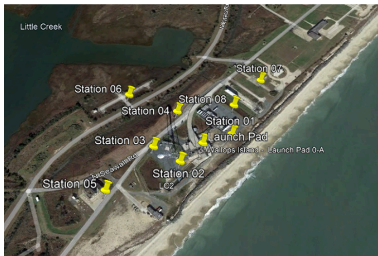
Figure 8: Map showing the locations of each of the microphone stations (Pumas) that collected data at the Antares 230 NG-19 rocket launch
