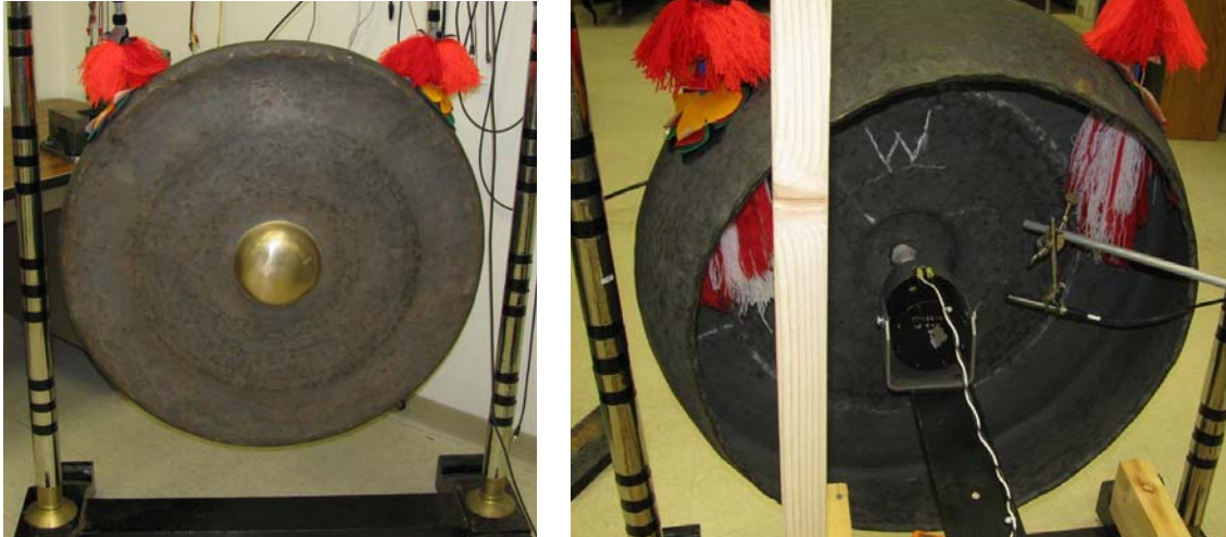
Figure 1: Left: The front of the gong, with the boss (the polished, raised dome at the center) visible. Right: Microphone placement behind the gong and the location of a shaker that was used for some tests to drive the gong continuously.
