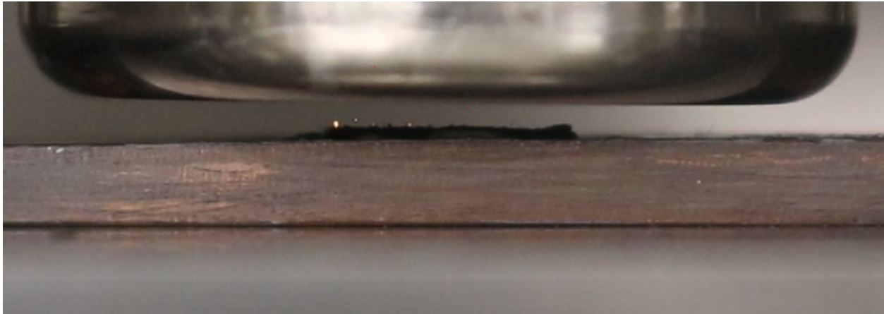
Figure 4.5 The 50 50 \mu\text{m} close to the electric field at failure ( 1.18 \text{ V}/\mu\text{m} ). Note the visible light emission from the outlier carbon nanotubes.
