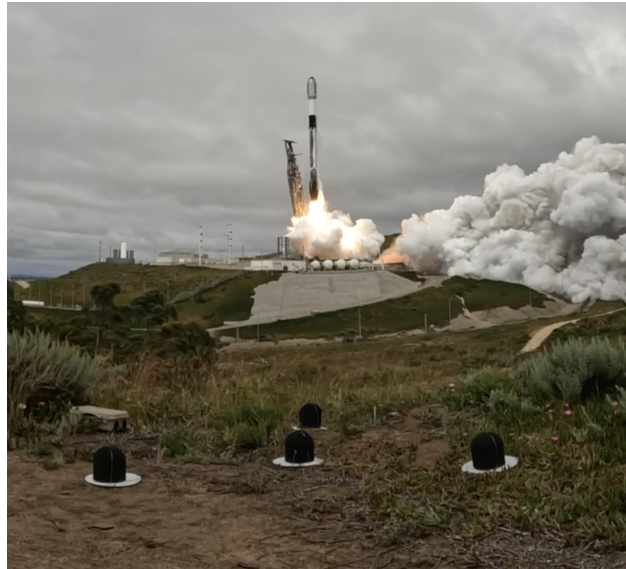
Figure 1.4 Transporter 8 mission launch aboard the Falcon 9 rocket on June 13, 2023, from Vandenberg Space Force Base. Ground-based acoustic recording equipment, in the form of a vector intensity probe, is deployed on site.
