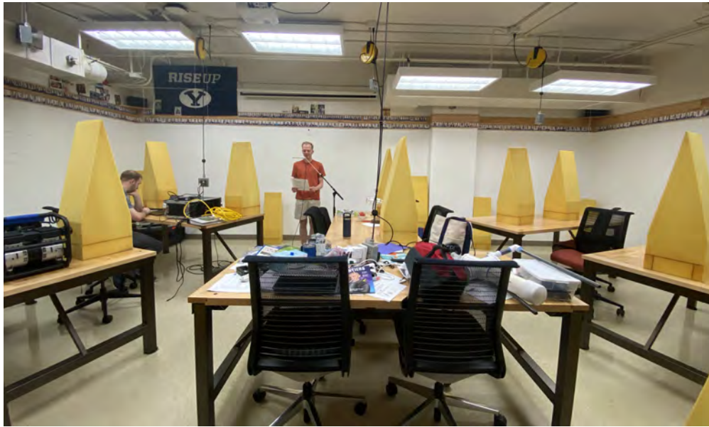
Figure 3.7 An image of vocal strain tests being administered in room N106. The participant is standing at the front of the classroom and spoke near an elevated microphone. Yellow foam wedges were placed around the room to decrease reverberation.
