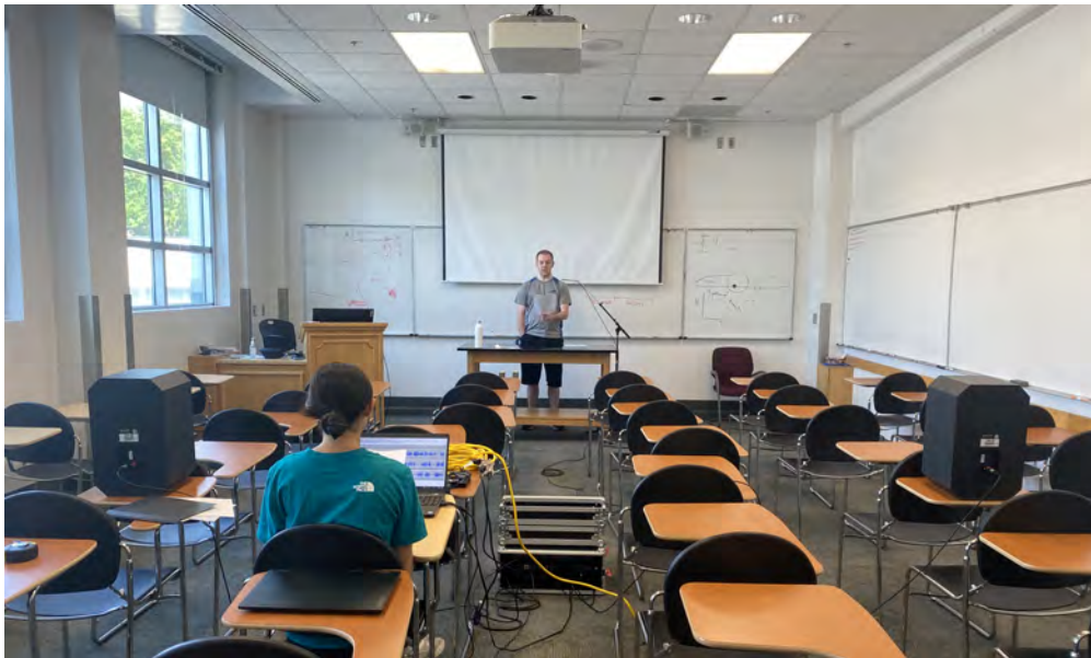
Figure 3.5 An image of vocal strain tests being administered in room C247. The participant is standing at the front of the classroom and spoke near an elevated microphone. Loudspeakers on both sides of the room output background noise at successively increased levels during testing.
