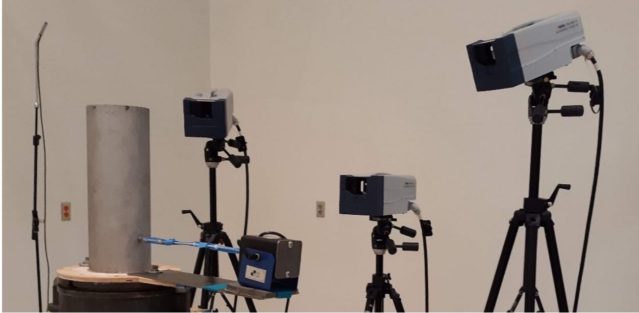
Figure 2.5: The cylinder setup for a 3D vibration measurement in BYU's large reverberation chamber.
