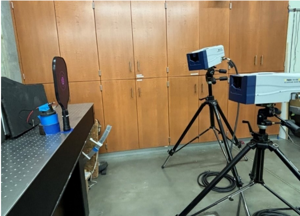
Figure 6.6: ( color online ) The SLDV experimental set up for the pickleball paddles.
