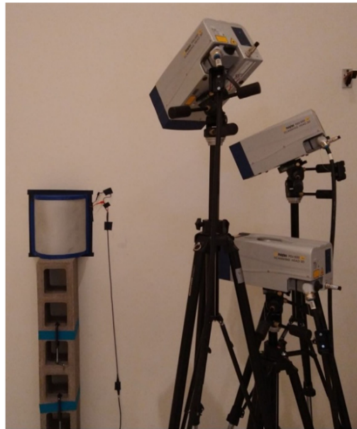
Fig. 2. An example of the 3D SLDV set up in a reverberation chamber prepared to scan a curved aluminum panel with a 0.16 m radius of curvature mounted in a steel frame and sealed to the wall acting as a baffle.
