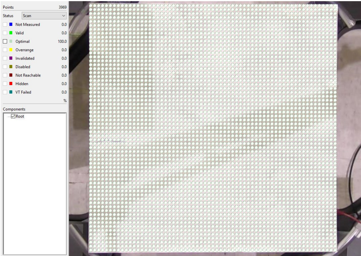
Figure 5.6: SLDV scan of the thin flat plate illustrating a 63x63 grid (~6.6 mm spacing).
