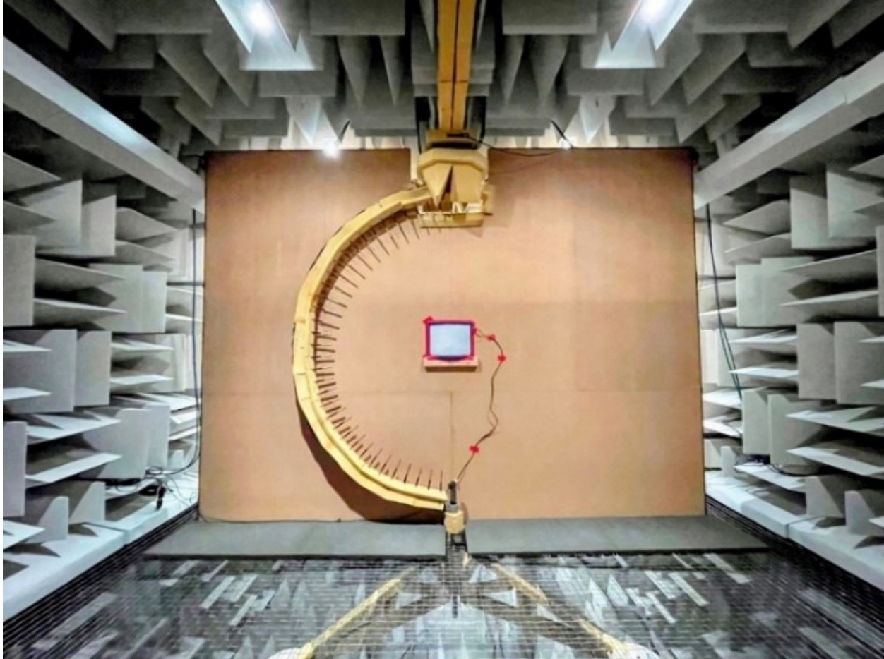
Figure 3.7: Experimental setup of the DMS (arc array) and wall inside an anechoic chamber.
