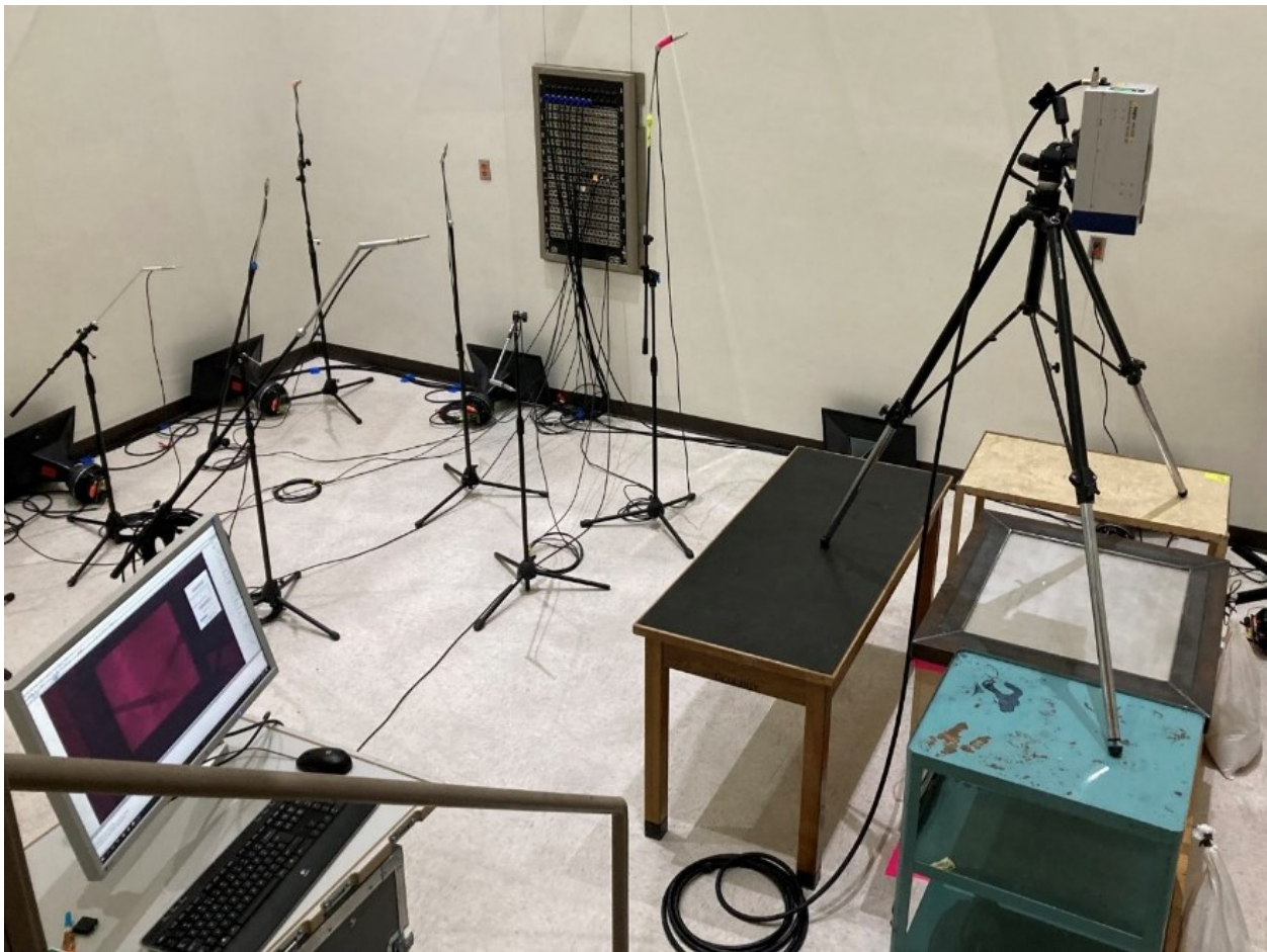
Figure 12.5: The microphones set up to take the ISO 3741 measurement and the absorption measurements with the experimental set up in the reverberation chamber.
