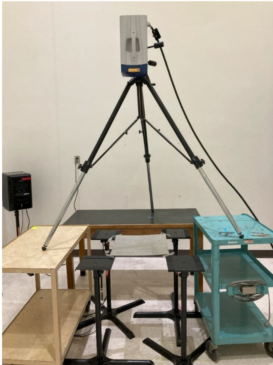
Figure 5.5: Flat plate setup for an SLDV scan in a reverberation chamber.
