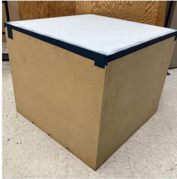
Figure 2. The mylar and MDF enclosure for I-VBSP measurements. There are three ports drilled in the bottom left to feed the source cabling. The bottom face is open so that the source can be enclosed on the floor where the source will then excite the mylar membrane acoustically. 8
