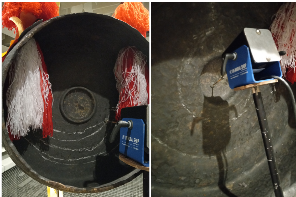
Figure B1 Examples of shaker positions for the original directivity study. On the left, the shaker is attached with putty to the side of the bebende in order to excite the mode shapes that have nodal lines through the center. On the right, the case where the shaker is positioned on the boss of the gong lanang to excite its axisymmetric modes is shown.
