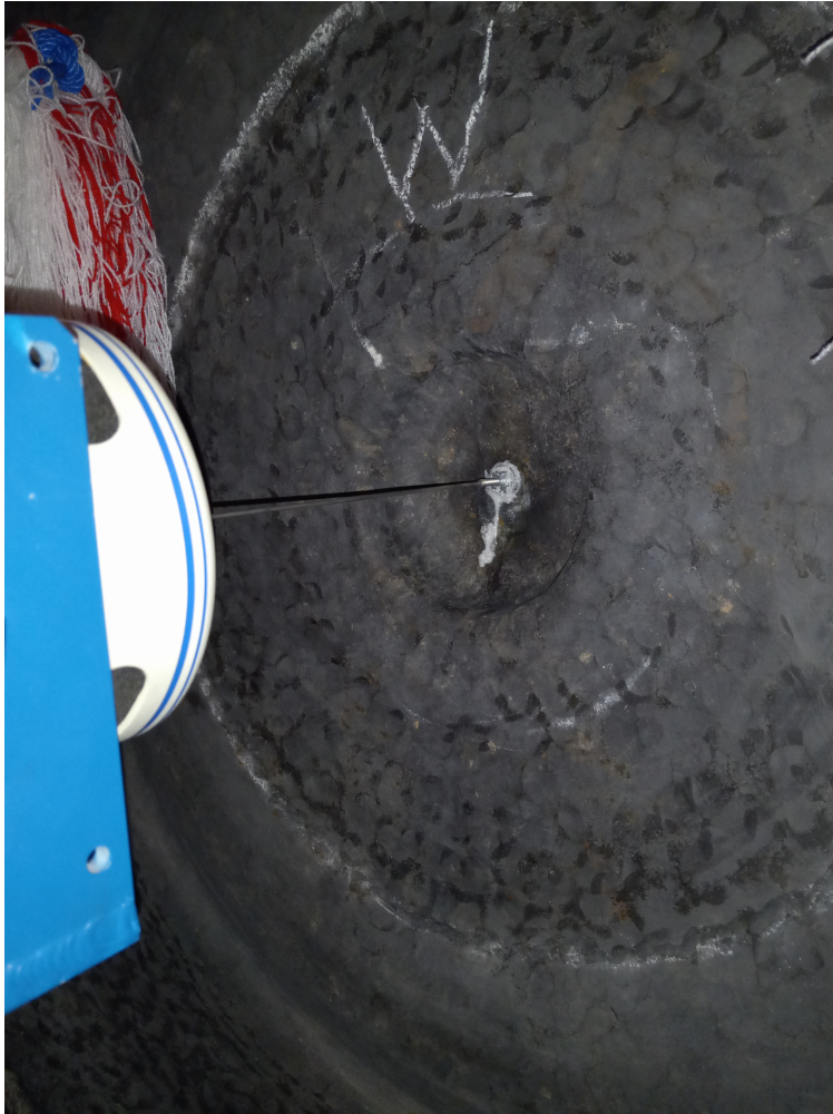
Figure B3 A single stinger piece connecting the shaker to the center of the gong wadon. The stinger rod ends in threading that was attached to a small round plate about the size of a nickel. This plate was then glued to the gong. The best stinger connection and position were achieved by setting the gong and shaker in the anechoic configuration seen in the left picture above. After gluing the stinger to the center of the gong, it would be pushed forward slightly to displace the gong before being tightened in place. The constant pressure from the weight of the gong would provide an adequately strong attachment for the higher amplitude tests.
