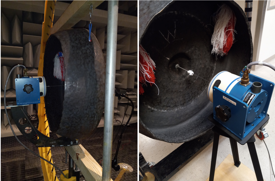
Figure B2 Two methods for mounting the shaker. The anechoic measurements required a stand that would not block the path of the rotating microphone array, so it attached directly to the frame underneath the gong as seen on the left. The stand on the right sits on the floor and can be adjusted to the desired height to center the stinger on the boss of the gong. This configuration was more convenient for SLDV measurements. In this image the stinger was comprised of two separate pieces connected by a threader piece. Any loosening of this piece would introduce noise to the system and white foam seen here was tied down to the piece to reduce the noise. Eventually this configuration was abandoned for a new stinger seen in the picture below.
