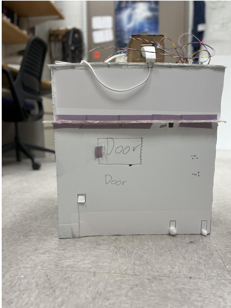
**Figure 2.2** Photograph of the front-facing side of the insulated heat box. The cut-out labeled “Door” provides an access point for observing or adjusting the optical experiment inside without removing the entire enclosure. Cotton insulation is visible at the some of the openings, helping seal gaps and improve thermal retention. Wiring from the fan and thermistor array exits through the top of the box.
