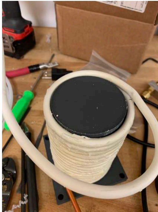
Figure 3.7 Custom copper solenoid used as the "dummy coil" in the ramp-up stage of the bias coil circuit. The solenoid carries both water and electrical current.
