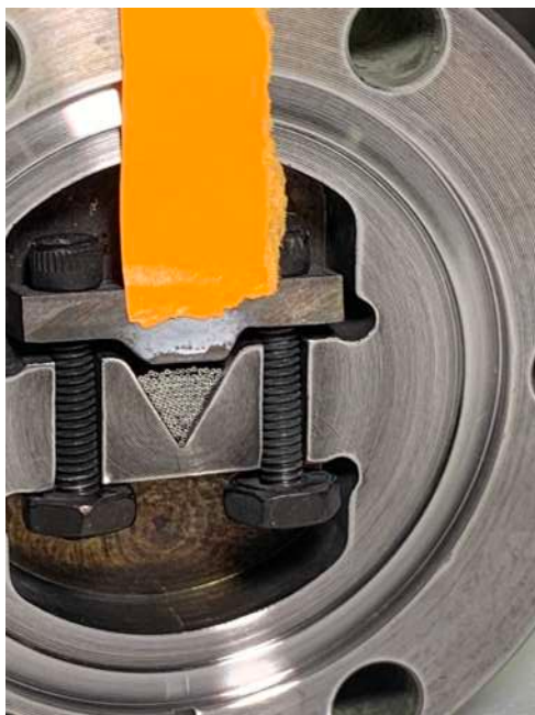
Figure 3.5 Close-up of the custom-made nozzle flange. The 120 small tubes in the nozzle had to be placed by hand.
