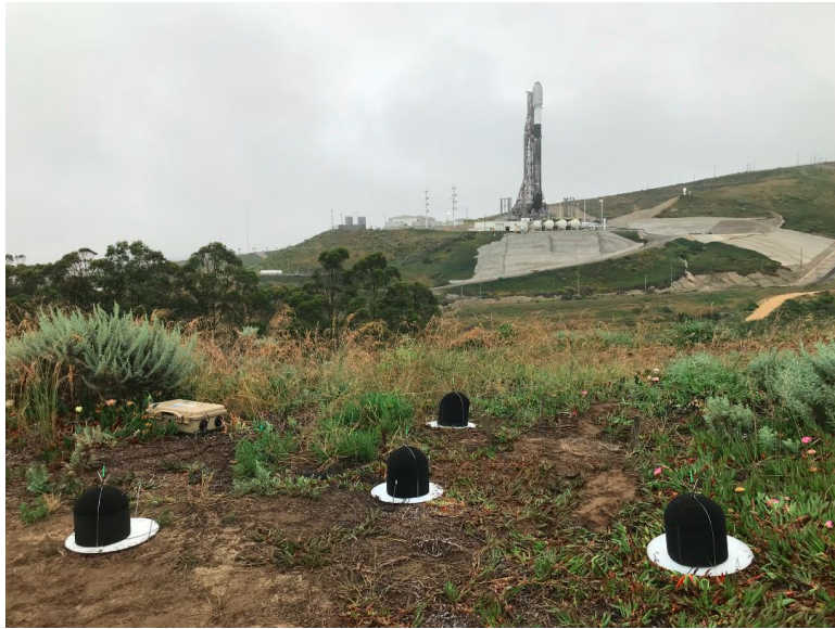
Figure 6.2 Example measurement setup near the launch pad. Although this station had four microphones, most stations used a single microphone.
