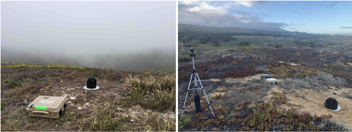
Figure 7.2 Example measurement station consisting of an inverted microphone placed over a hard plastic ground plate and covered by a dome windscreen, with all other electronics placed inside a weather-resistant case. Some locations also included small weather stations mounted on tripods.
