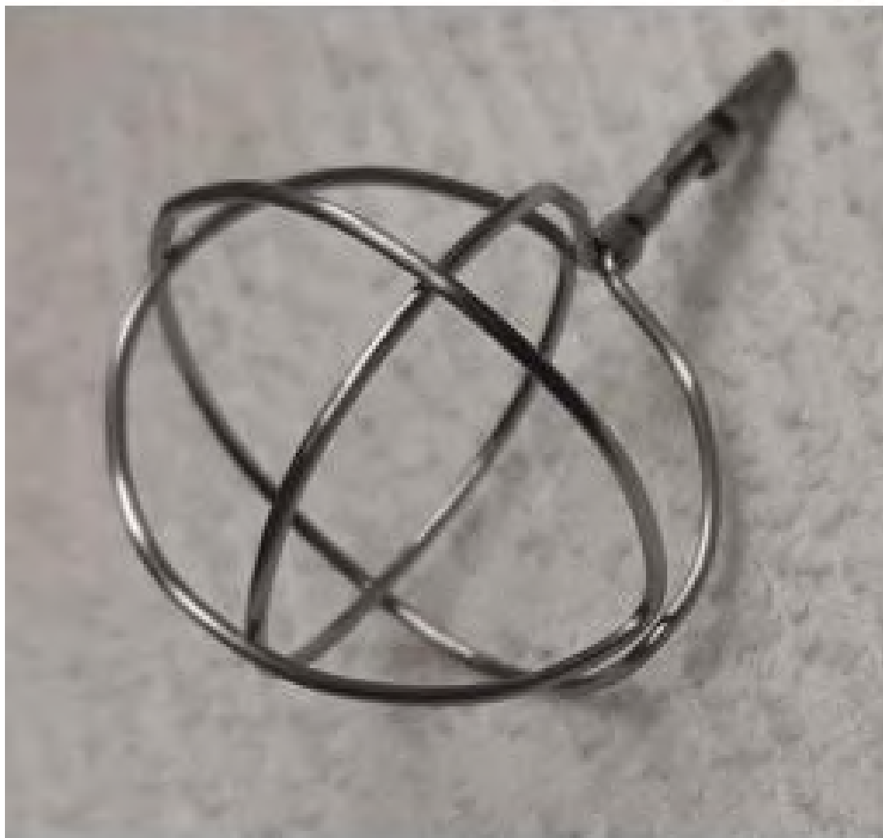
Figure J.3 Photograph of the smaller stainless-steel cathode grid.
