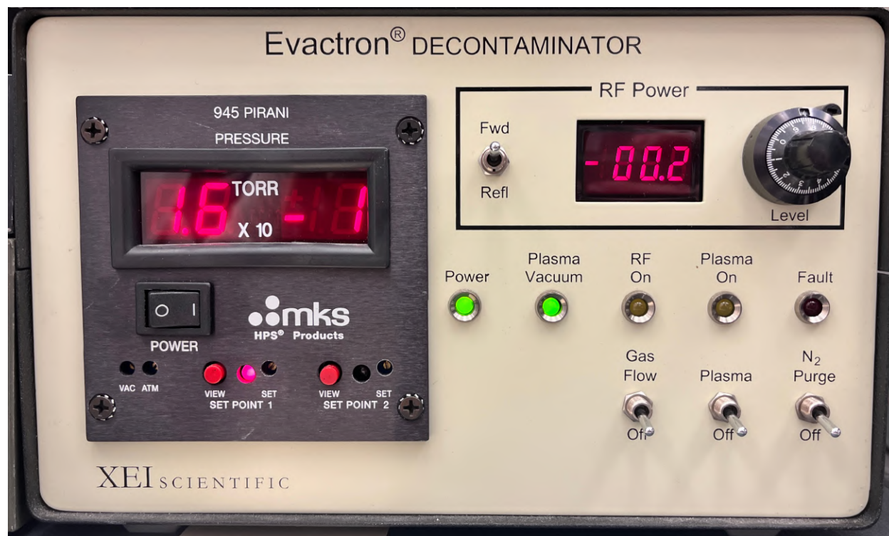
Figure 4.7 Photograph of the Evactron DECONTAMINATOR unit. This unit is used to control the plasma ignition instrumentation. This includes a toggle switch for gas flow, a plasma ignition switch, and an adjustable power output with live readout of the RF power measured.
