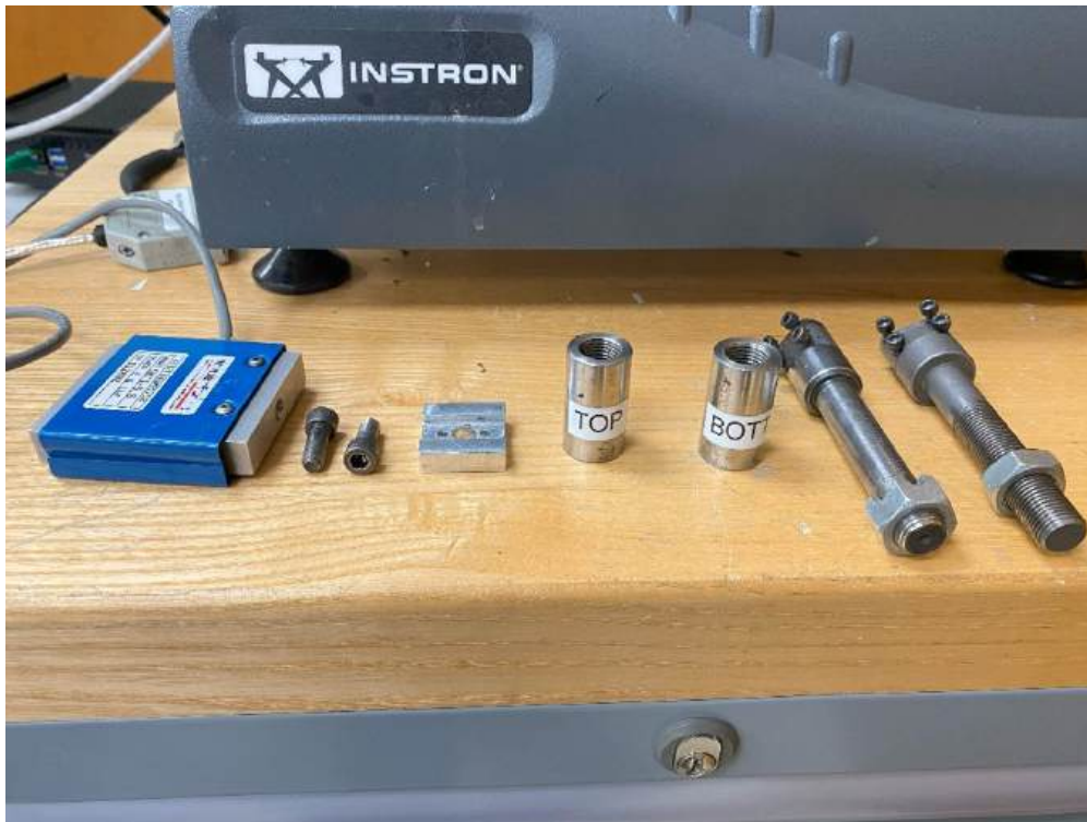
Figure A.1 From left to right: 5.6lb load cell, two small bolts, spacer, threaded top/bottom clamp holders, threaded top/bottom clamps
