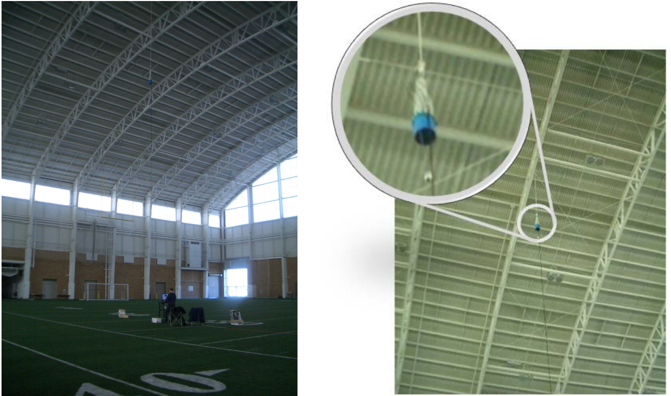
Figure 2.2 On the left is a wide view of the setup inside the indoor practice field. This shows how large the building is. On the right is a close-up of the detector and source configuration. We oriented the detector so the incident neutrons were directed at the flat side.
