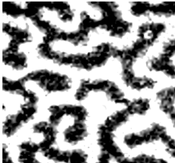
Figure 2.2 XRM image of magnetic domains in the magnetic thin film. Perpendicular anisotropy leads to a striped domain configuration when the net magnetization is zero. Image size is about 1\mu\text{m} \times 1\mu\text{m} .
