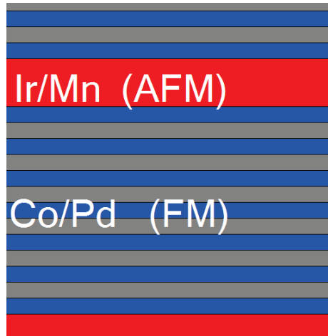
Figure 1.4 Exchange-bias Multilayer An example of an exchange-bias multilayer. In our [[Co(4\text{\AA})/Pd(7\text{\AA})]_{12}IrMn(24\text{\AA})]_4 films, an antiferromagnetic Ir/Mn alloy layer is periodically inserted into a repeating ferromagnetic Co/Pd multilayer. Exchange coupling occurs at the interface between the ferromagnetic and antiferromagnetic layers, causing uncompensated spins in the antiferromagnetic material very near the interface.
