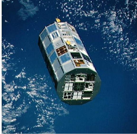
Figure 1.2 NASA's LDEF satellite as seen from orbit. It was used to study the effects of long-term exposure to the environment of space on various materials. Image retrieved from http://www.astronautix.com/graphics/0/10061447.jpg
