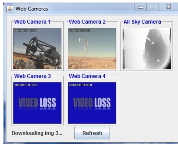
Figure 3.5 The web camera interface. Initially, the displayed images are buffered images and should not be taken as accurate. Click the "Refresh" button to begin downloading current web camera images. Click on an image to display a larger version.
