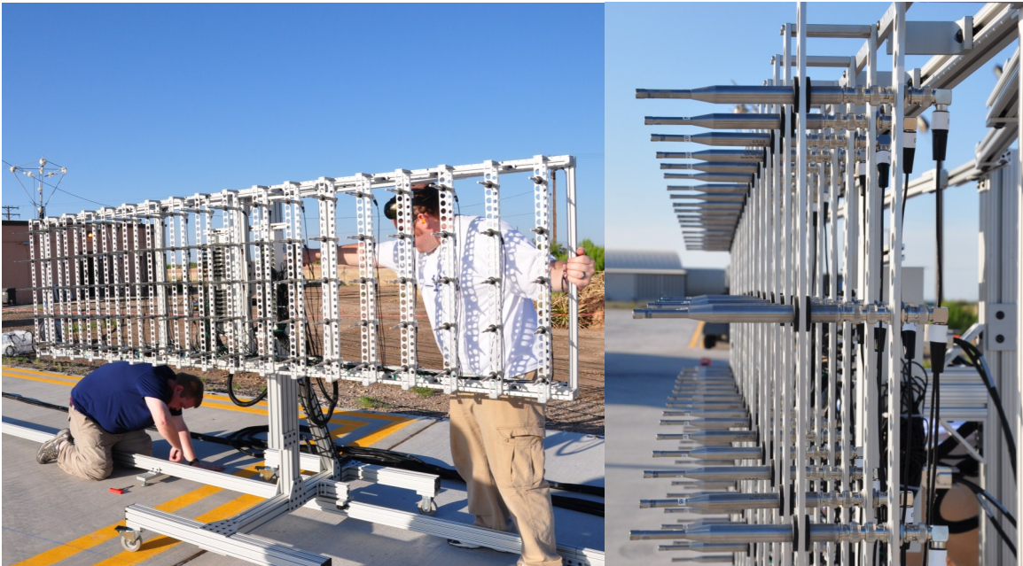
Figure 1.3 A close up of the rig; a rectangular 5 by 18 microphone array. The rig is movable along a track.
