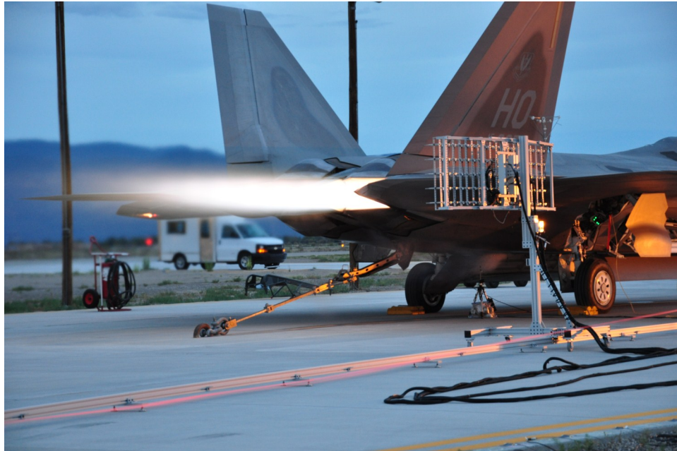
Figure 1.2 The jet strapped down to the runway with a rig of microphones to take data.
