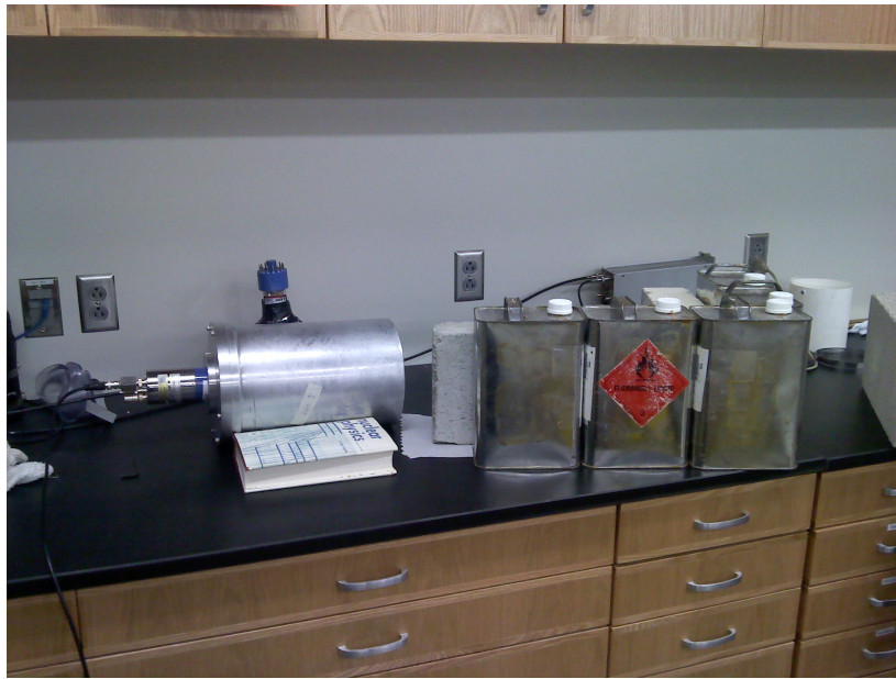
Figure 2.6 The combination detector inside the light-tight can is placed 8 cm away from the source. Cement blocks and cans of water were placed around the source for personnel shielding.
