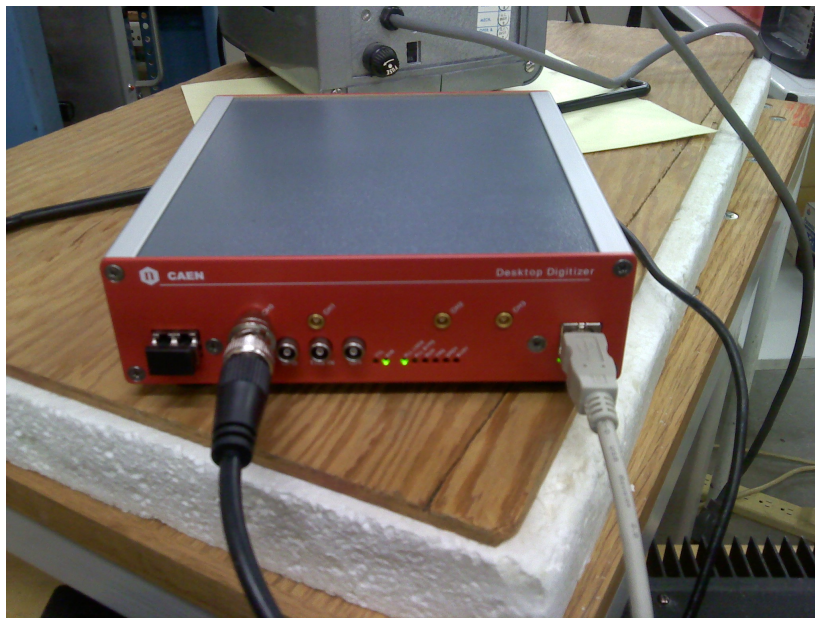
Figure 2.7 The digitizer takes the voltage from the detector and converts it to a digital signal.
