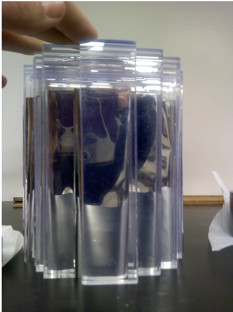
Figure 2.4 The cadmium sheets are sandwiched between the layers of plastic.
