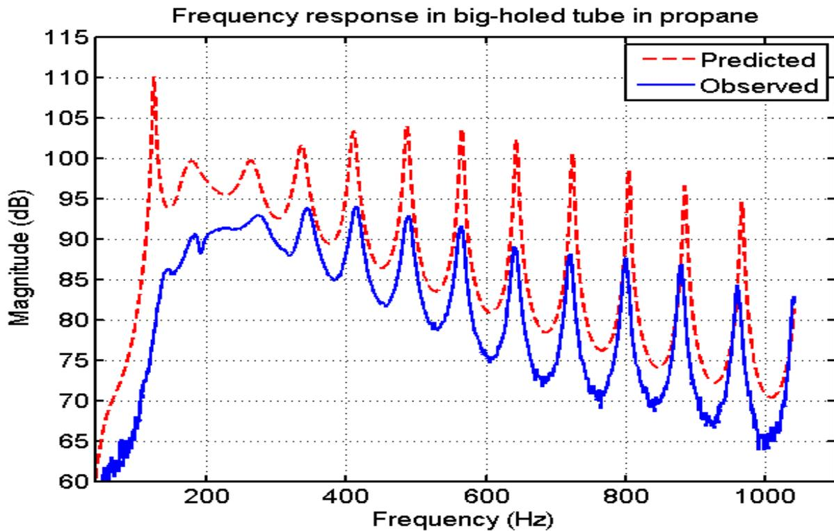
**Figure 8** Frequency response at the cap end of tube comparing the observed response (tube in operation) to the model predicted response in big-holed tube.
