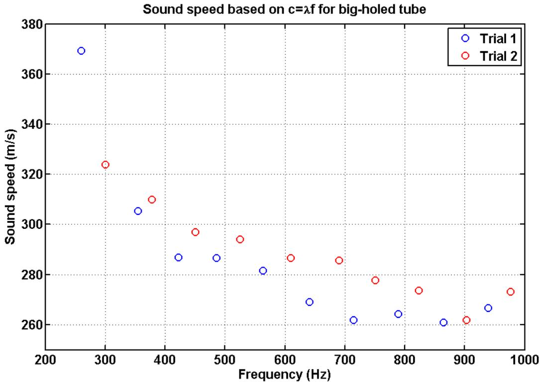
**Figure 10** Calculated sound speed versus frequency using  $c = \lambda f$ . The distance between flame peaks is used to calculate  $\lambda$  and the frequency input into the tube from the signal generator is used for  $f$ .
