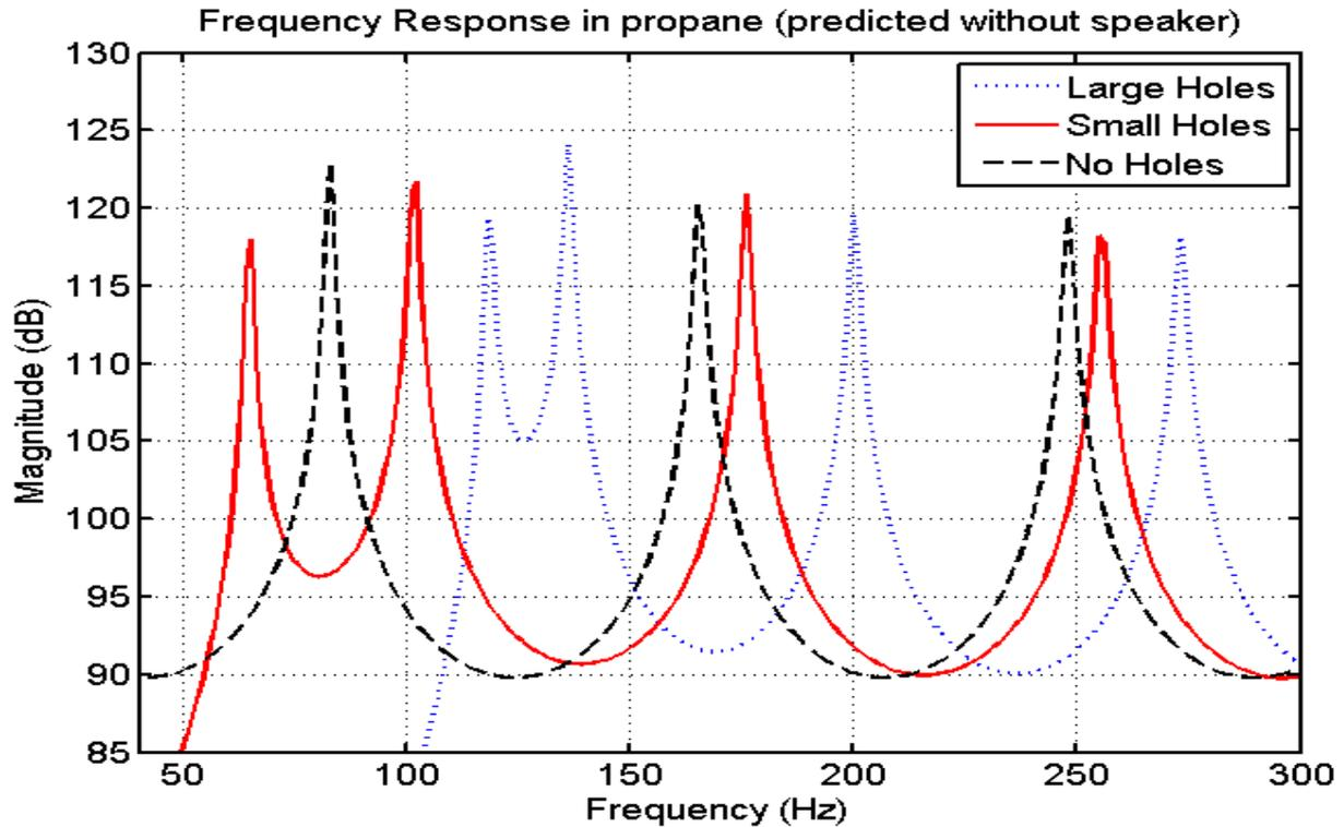
**Figure 7** Model predicted frequency response at cap end for three cases of the tube: no holes, small holes, and large holes.
