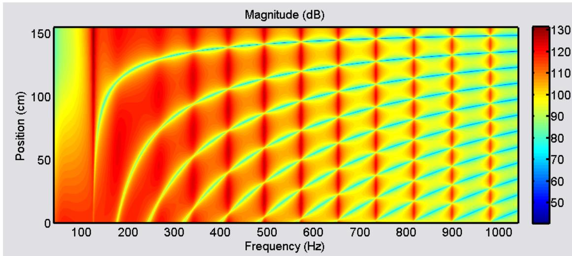
**Figure 5** Graph of dB magnitude of pressure inside the tube from the speaker end (0 cm) to the cap end (150 cm) looking at frequencies from 40 Hz to 1040 Hz. The graph is modeled *with* the source.
