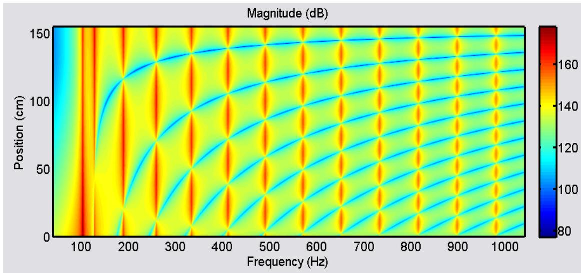
**Figure 6** Graph of dB magnitude of pressure inside the tube from the speaker end (0 cm) to the cap end (150 cm) looking at frequencies from 40 Hz to 1040 Hz. The graph is modeled *without* the source but *with* the source cavity.
