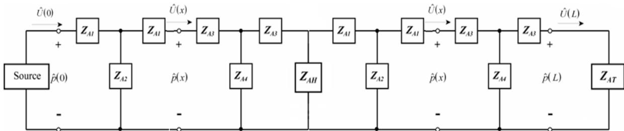
**Figure 2** Waveguide circuit diagram for a tube with source, termination, and one hole ( $Z_{AH}$ ).
