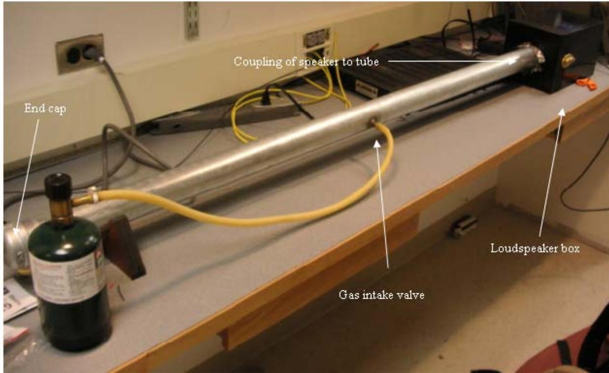
**Figure 3** Flame tube setup.
