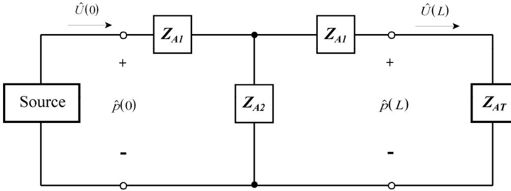
**Figure 1** T-network with source and termination ( $Z_{AT}$ ).
