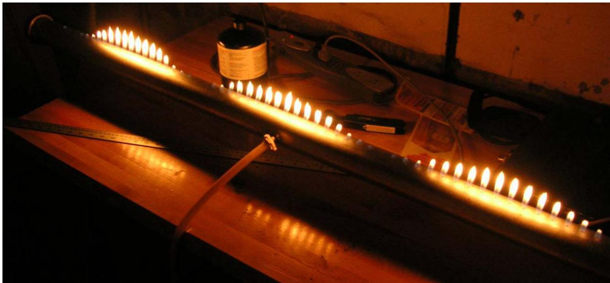
**Figure 4** Flame tube in operation.
