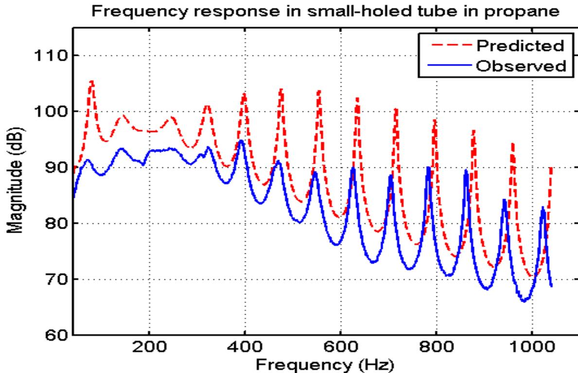
**Figure 9** Frequency response at the cap end of tube comparing the observed response (tube in operation) to the model predicted response in small-holed tube.
