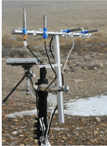
Figure 2.1 Station 3 rig showing the microphone holder
