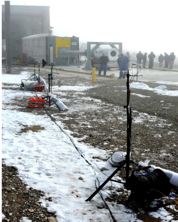
Figure 2.8 The KEI Stage 2 rocket motor, test pad, test bay and microphone stations. Station 1 is the station nearest the motor. The next station is Station 2, followed by the weather station and the station nearest the camera is Station 3.
