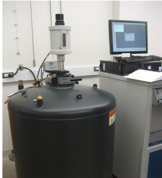
Figure 2.1 Picture of our VSM instrument: A black cylinder contains a superconducting magnet, and the attachment top of it is the linear motor for vertical motion.
