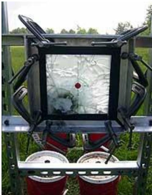
Figure 12 AFRL Ballistic Testing set up. This test was conducted with ballistic ALON manufactured according to the licensed process owned by the Surmet Corporation
