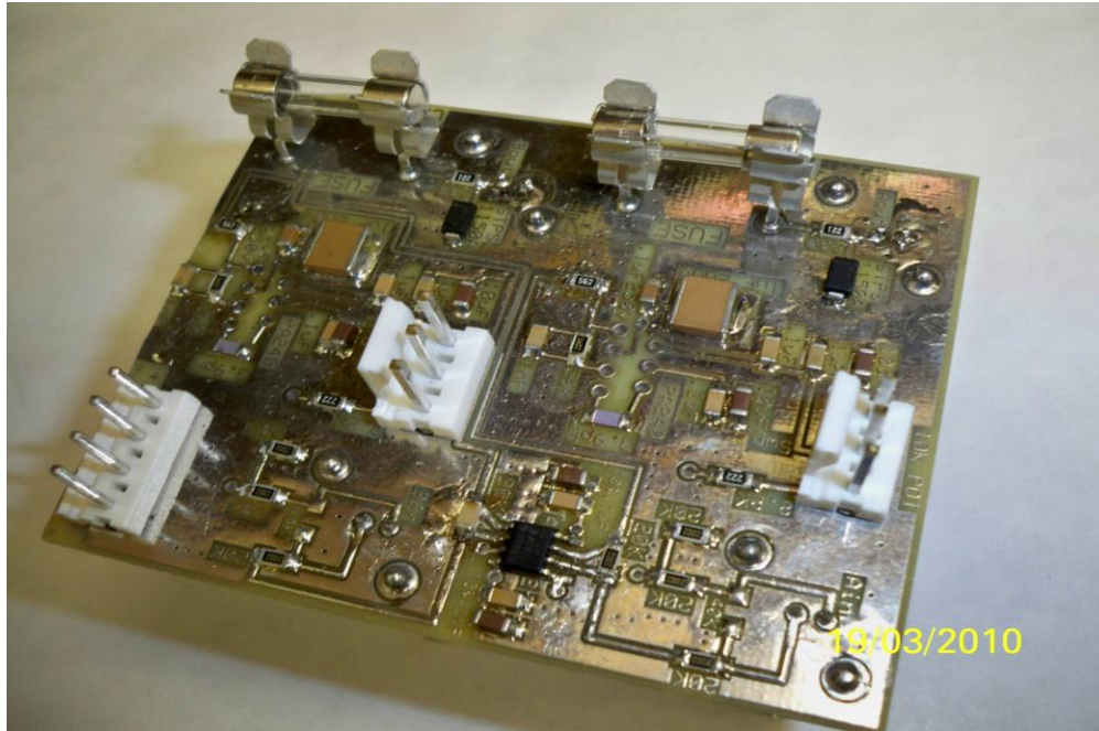
Fig. 2- Photograph of the piezoelectric driver using surface mount components
