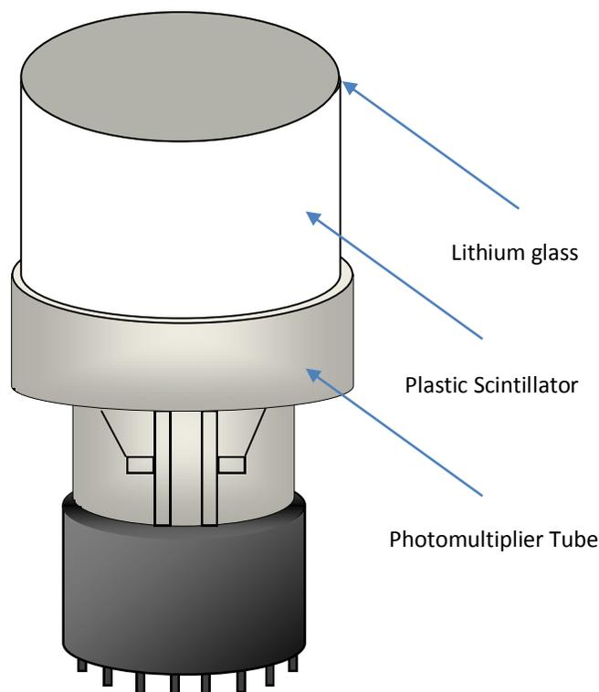
**Figure 1.1** Lithium Glass Neutron Detector
