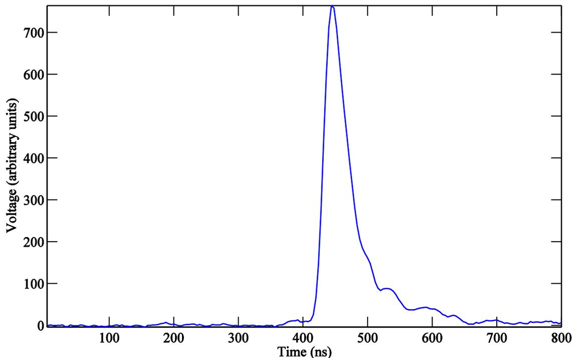
**Figure 2.2** A Typical EJ 212 Pulse
