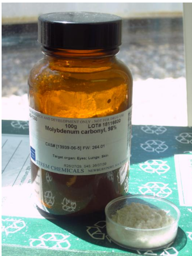
Figure 1.3 Molybdenum Carbonyl ( \text{Mo}(\text{CO})_6 ). Above we see a perspective drawing of a \text{Mo}(\text{CO})_6 molecule showing its octahedral structure, with a molybdenum atom in the center and six carbon monoxide molecules at its octahedral sites (image taken from Wikipedia ). To the right is a photograph taken of a bottle of \text{Mo}(\text{CO})_6 , and in the petri dish we see \text{Mo}(\text{CO})_6 in its powder form.
