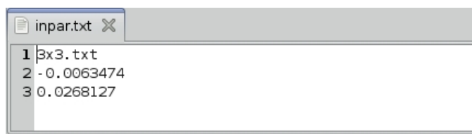
Figure 3.1 Input file for nicpsf . First line - the file that contains the 3 \times 3 array from the original image. Second line - background value ( msky ) obtained from the original phot operation. Third line - stdev obtained from the original phot operation.
