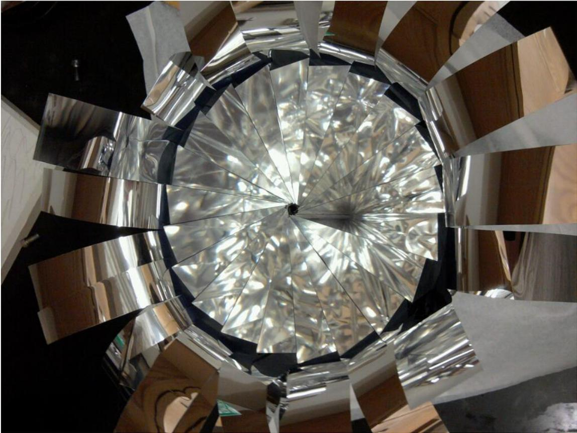
**Figure 3.2** Final construction of wedge detector
