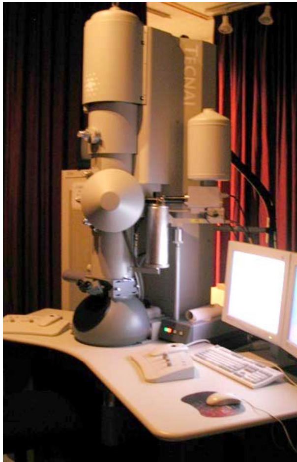
Figure 1.1 A Tecnai F20 Analytical STEM, similar to the TEM used to analyze our grids.
