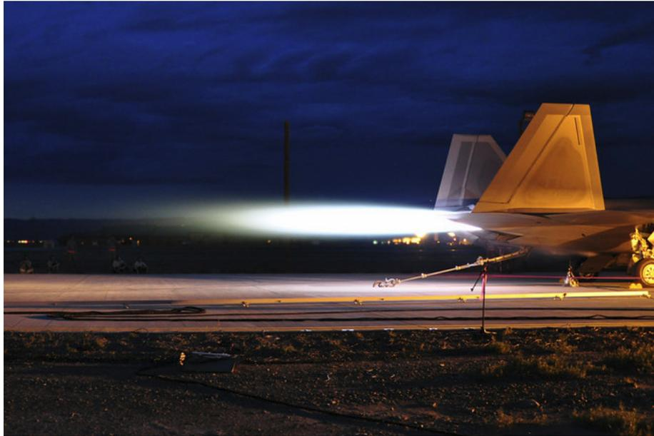
FIG. A.1. Photograph of an F-22 Raptor held on the ground for acoustics testing.
