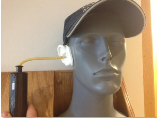
Figure 2.3.1 - a GRAS 114 dBA 1 kHz Calibrator fixed in the ear of the E.A.R.S. mannequin.
