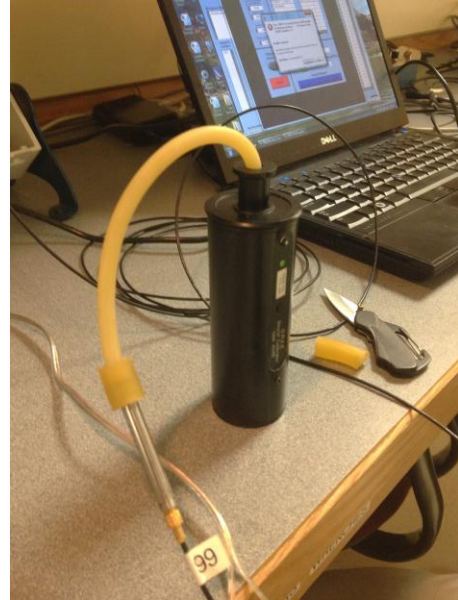
Figure 2.3.2 - 1/4" Condenser Microphone connected to the GRAS calibrator measuring its sensitivity via the surgical tube.
