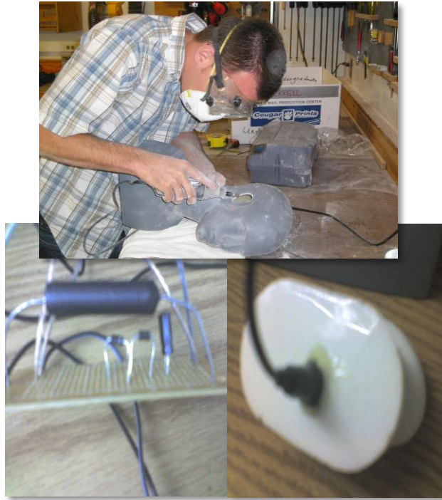
Figure 2.1.1 – The construction of the E.A.R.S. mannequin with microphone ear and voltage divider featured.
