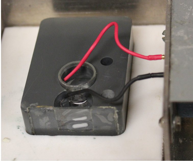
Figure 3: Experimental setup of the nystatin/ergosterol fusion assay. 150 mM KCl buffer was added to both the inside of the cup and the front chamber. Ag/AgCl electrodes are immersed in the solution in the front and back chambers. The front chamber contains a stir bar to mix the osmotic gradient and vesicles.
