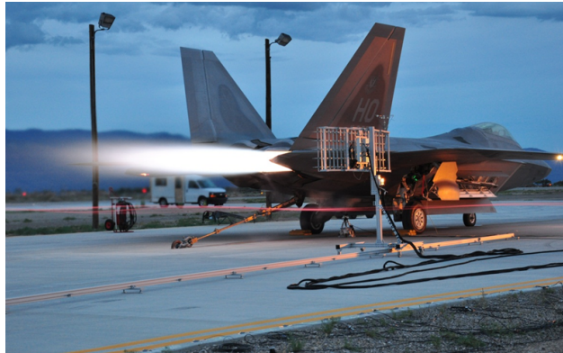
Figure 1.1 The tethered F-22 with one active engine. The microphone rig is also visible.
