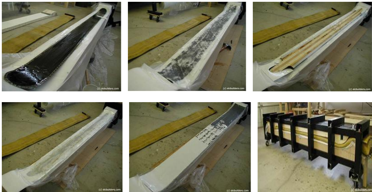
Figure 7: Steps of making a ski (Leang, Leang, & Wu, 2007)
