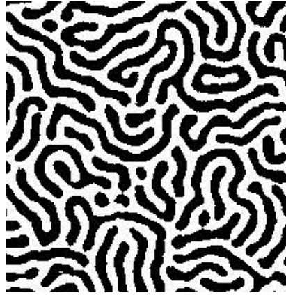
Figure 3.10 Co-Pt thin film, under no external magnetic field influence, forms maze-like magnetic domain patterns.[Westover, personal communication]
