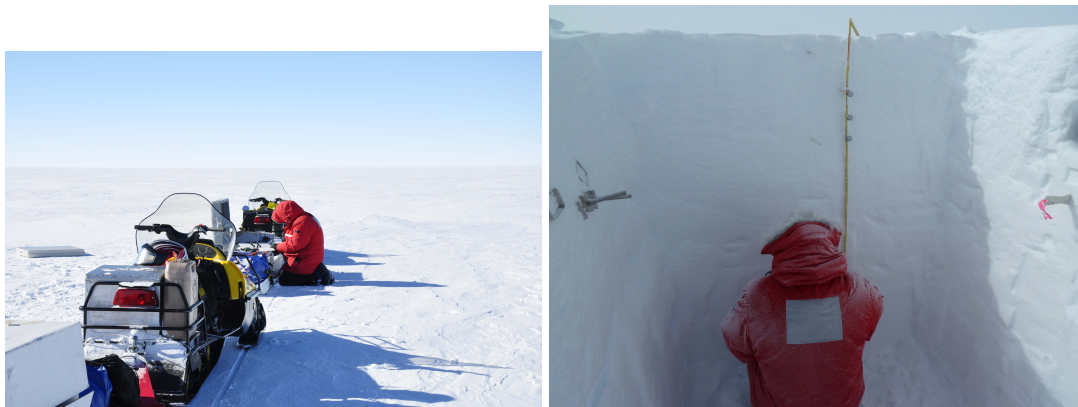
(a) Snowmobiles used to traverse Antarctica. (b) Snow pit used to obtain SMB measurements.
