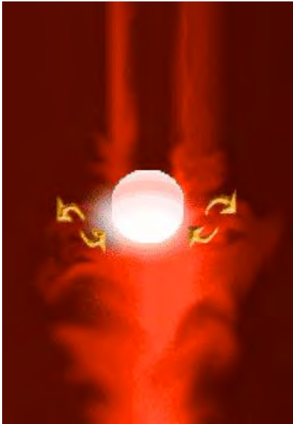
Figure 1.3: Convection currents push up on a particle to support its levitation. [6]
