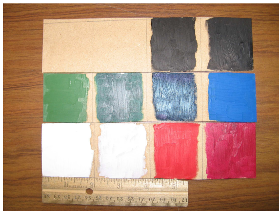
Figure 2.3 Photo of single-color targets for external-beam analysis
