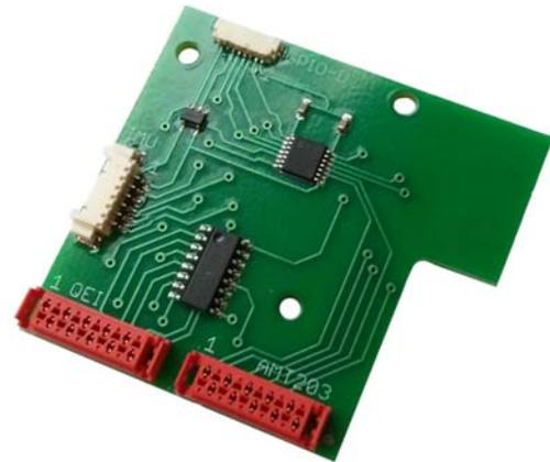
**Figure 10: AMT203 Encoder Interface Board**
