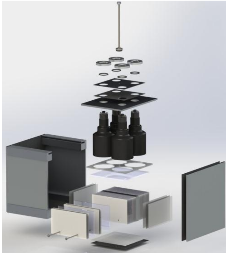
Figure 2.2 An exploded view of the detector. The detector consists of 4 photomultiplier tubes to detect the light from the detection medium and 21 sheets of plastic scintillator with cadmium foil and aluminized-Mylar inbetween each sheet of plastic. The aluminized-Mylar helps the light reflect and ensure as much light as possible reaches the PMTs. The PMTs and the detection material are held in a light-tight aluminium box.
